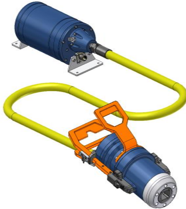
Figure 2: Electrical Torque Tool powered by EPC
